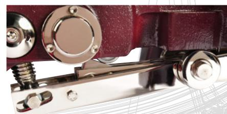
Split Rocker Arm: Split construction reduces pressure on the frame. Unique Dresden System version eliminates the need for a transfer bar.
