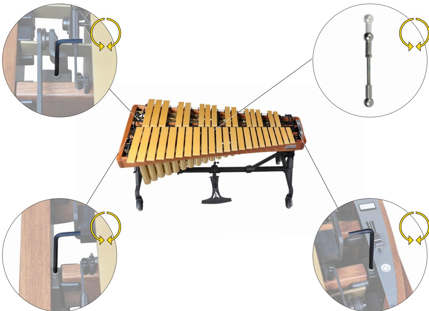
As the dampening felt wears, the adjustable dampening system can extend the life of the felt before replacement is necessary. Increase the length of the threaded connection piece to apply more pressure against the bars, and then adjust Rail 2 as described in Steps 5.3-5.6 of "Install bars and adjust dampening mechanism."
